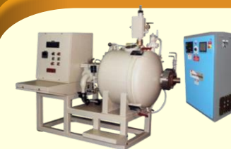
High-Vacuum Induction Melting-Casting System
