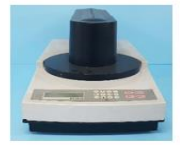
4-point probe for nanofilms
